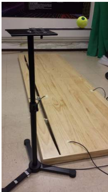
Figure 10: Experimental set-up: an adjustable stand for speakers, with a transverse metal bar, and a tennis ball
