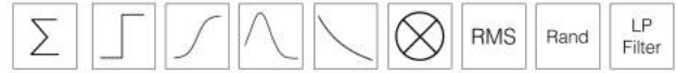
Figure 1. Graphical symbols used for the schematic representation of network nodes and connections. From left to right: summation, threshold function, sigmoid transfer function, gaussian transfer function, negative exponential function, gain function, root mean square (RMS), random number generator, low pass filter.
