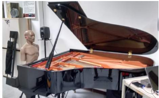
Figure 3. The recording setup. Left: block scheme of the acquisition chain. Right: a picture of the KEMAR mannequin positioned at the pianist location. The setup was moved to the center of the room for the recording session.
