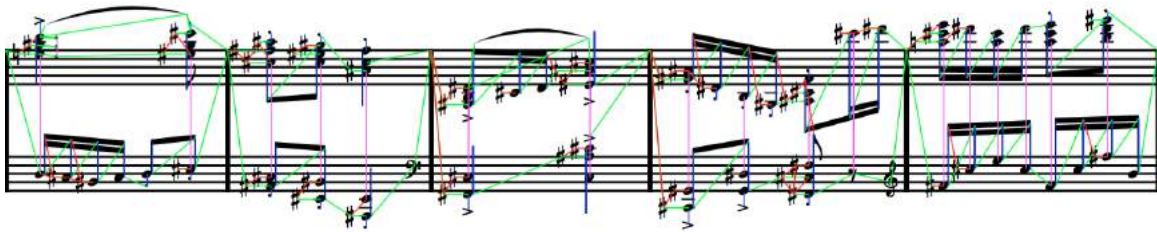
Figure 2. Graph showing the types of edges between the vertices. Green : Soft horizontal edges (quadratic term); Blue : Soft vertical edges (quadratic term); Magenta : Hard Edges (equality constraint); Red : Conflict edges (inequality constraint).
