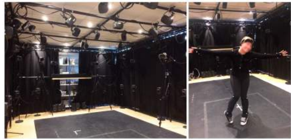
Figure 4. Lab set-up for the Experiment with 21 markers positioned on the body. 8 Motion capture cameras are hanging on the walls.
